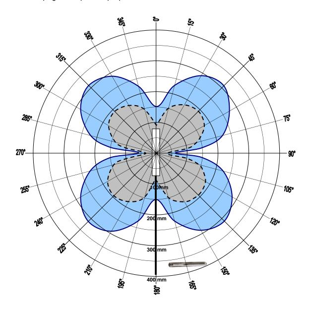
reading no metal in the surrounding area – antenna is adjusted
